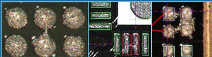
Low Solder Bridge Inspection
