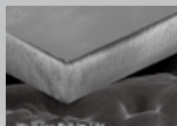
[GaAs] SEMx300 140mm/s 1pass 100 μm
